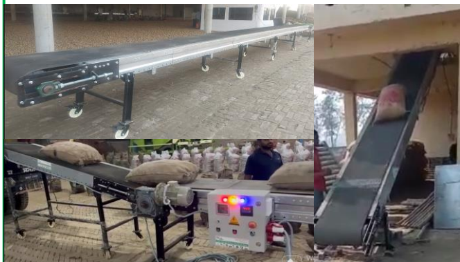
Conveyor profile with rough top belt.
